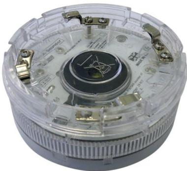
The sandwich sounder has no wiring to connect as it just clips straight on to a standard base. It will run as a platform sounder using no address, it is controlled by the detector fitted to it. It can also be given an address via the handheld programming tool making it an addressable sounder.
