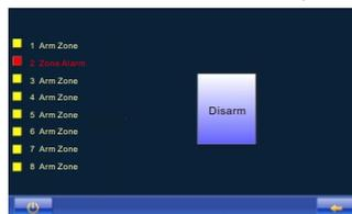
Tenant can check and cancel the alarm by door phones. Press “disarm” on the alarm interface, if it is express mode, disarm by express mode. If it is separate control zone, disarm by separate mode
