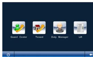
Guard Center : Call and talk with Guard Center, Calling sequence is Guard Station, back up Guard Station, Guard Center, back up Guard Center. If there is no answer, it will cut off automatically. If answer in the setting time, max conversation time is 120s. The tenant could delegate Guard Center to execute the service.
