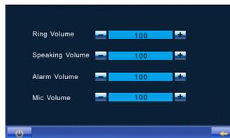
Touch “Volume”. There are 5 levels of Volume, press “+” to turn up the volume, press “-” to turn down the volume. Press ← to save the data and return to the previous menu.
