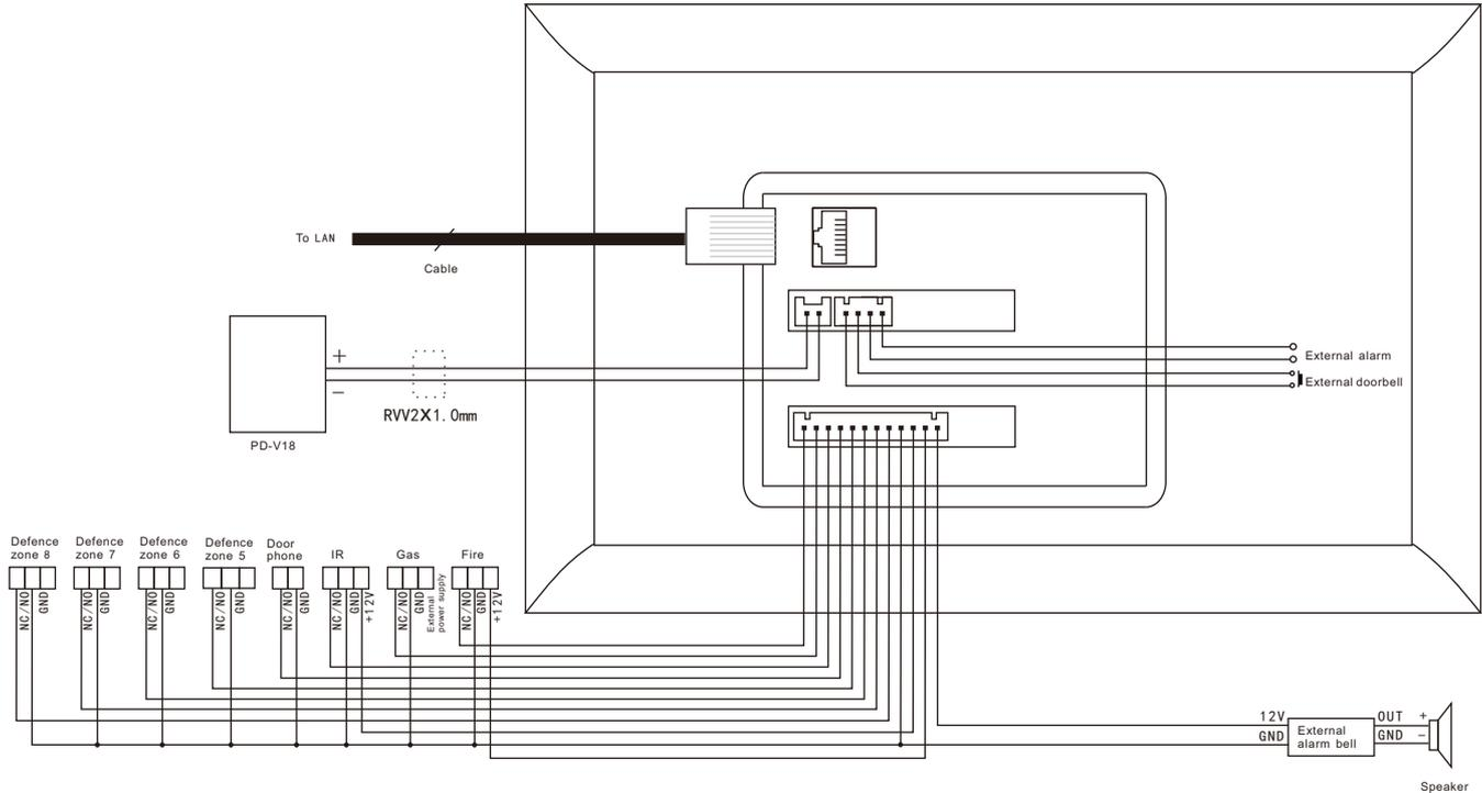
1. Defence Zone 1~4 can connect the short circuit or open circuit sensor, but could not be connected to the pulse signal probe as the switching signal time is more than 200 millisecond.
