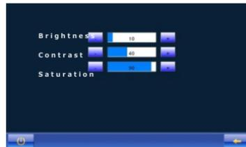
There are totally 100 levels, press "+" can turn up, or "-" to turn down, press "←" to save the data and go to the previous.
