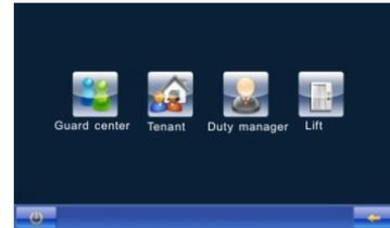
5.2.1 Call Guard center: This function is calling the Control Center. If no answer, it will cut off automatically, or else the call can be kept in 2 mins, and click " " to hang up.
