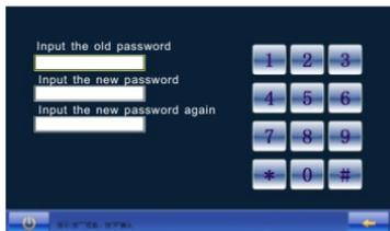
Input the old password( input the "88888888" for first usage), and press "#" to confirm it. If wrong, the display will prompt, then click "Ok" to re-enter the old password, and click "cancel" to return to the main menu. In the case of right old password can automatically activate the new password input box. Tenant may be prompted to enter a new password continuously, and press "#" to confirm, click "Ok" to change the password for the new password, press "←" to return to the previous menu.
