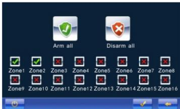
Click the arm zone you need, and press " ✓", " ✓ " means arm is enable, " x " means arm is disable, click " ✓ " again to confirm. If "toot" sound is heard, the alarm LED turns to be yellow.
