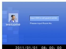
The Gate Station works after all parameters are correct. Press "\*" first, then press "#", and release the two keys at the same time, The screen will show:
