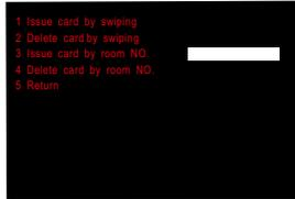
Input 6 digits (3-digit floor NO.+ 3-digit room NO.,for example 001001) the room NO.of tenant. Press"#”again, then swipe the card at induction zone,it means issued successfully.the user could continue inputting other room NO. to issue other cards.Press “\*” to return to previous menu.
