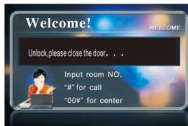
If the device is Gate Station, tenant can use special password to unlock. The method is to input " \* " Room NO. + password + " #".
