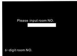
Input room NO. (Former 3-digit is floor NO., last 3-digit is room NO.), press "#" to confirm, the screen shows:
