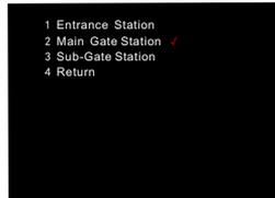
Press the device you want(" ✓" means selected),press"# " to confirm,the screen will prompt modify successfully.Press"\*" to return to previous menu.
