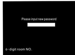
Input 6 digits new password, press "#" to confirm. Then the screen prompts to confirm special password again, tenant input new password again, press "#" to confirm. If entered two new special passwords are the same, it will prompt that new special password is modified successfully.
