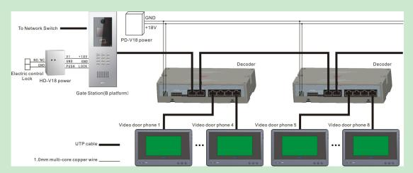
When the distance from door phone to decoder over 20 meters,so it should be added a power supply wire,as follows:
