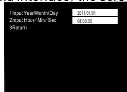
Press number keys to clear up the data in the input box, input the date and time, press "#" to confirm after finished, the screen will prompt modified successfully, it means the group data set successfully.
