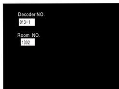
Thus, the first port of the decoder 13 had been modified to room NO.0109. Then input "0131 0110" (or press"#", input "0110" after moved the cursor 4 digits, following the same),"0132 0111", "0133 0112", modify the room NO. which correspond to output ports 2-4 to 0110-0112.Then modify the room NO. which correspond to output ports 5-8 to 0209-0212.
