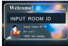
The Gate Station works after all parameters are correct. Press "\*" first, then press "1", and release the two keys at the same time, The screen will show:
