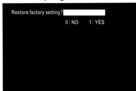
Press "1", then press "#", all the settings are initialized, Gate Station will restart automatically.
